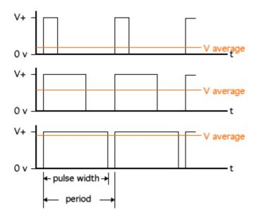
By using Arduino's analogWrite(pin, value) function we can vary the value of the duty cycle of pin's output. Note that the pin must be put into output mode and the value must be between 0 (0V) and 255 (5V). Any value in between will simulate a proportional intermediate analog output.
