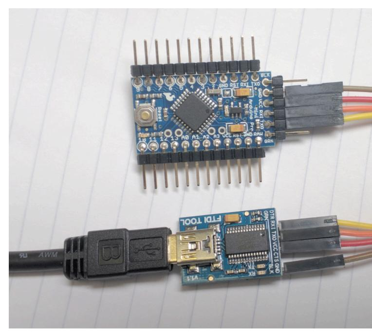
You will have to provide power separately to the Arduino because the debugger will not power it. This can be done on the Pro Mini through the FTDI board as shown above, or with a USB cable or AC adaptor on the Uno.
